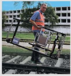
Weight of the assembled flaw detector does not exceed 22 kg. Overall dimensions of the assembled flaw detector are not more than: width - 900 mm; length - 1730 mm; height - 350 mm
