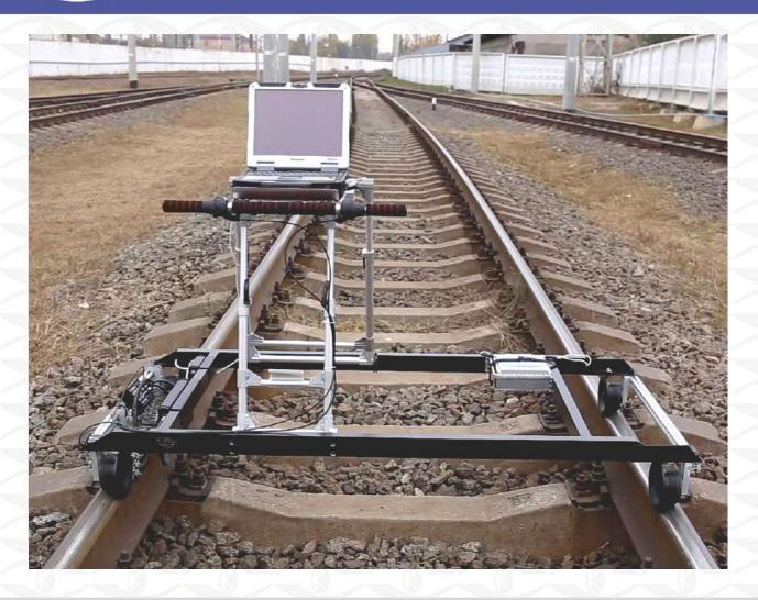
ETS2-77 eddy current single rail flaw detector is a mechanized scanner which is intended for manual eddy current inspection of rail head's active face and running surface of rails laid down in a track, for the presence of surface cracks. The flaw detector serves for detection of flaws, e.g. cracks in the rail head, as well as for evaluation of their depth.
