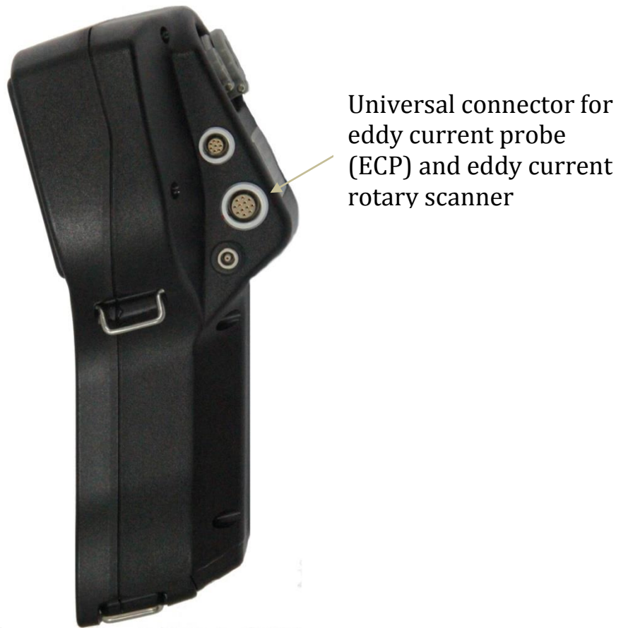
FIGURE 14 – Eddycon C eddy current flaw detector. Right side panel
