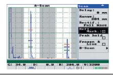
"REFLECTIONS MARKING" mode helps to imagine the detected defect location in the testing item in the same direction as ultrasonic beams (straight and multiple-reflected beam).
