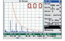
UD3-71 flaw detector distinctive feature is the measurement of equivalent defects dimensions. Using DGS diagrams UD3-71 flaw detector RF SIGNAL
