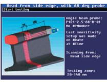
This mode is applied for solving special-purpose tasks. For example, when testing various single-type parts or when the part has many testing area. For solving this task "Special program interface" system is used in UD3-71. The necessary standard setups and program interface of "Special program interface" enter flaw detector from PC. The input setups are protected from illegal change by NDT inspector (operator).
