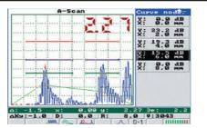
TCG level is set up in the point grid connected by linear sections, i.e. it is possible to set sundry TCG curve forms - piecewise-linear, step etc. TCG level corresponds to the signal attenuation in the given point relative to the set gain value. This option allows to test long-length items and items made from materials with great attenuation, it is also used for sensitivity setup when testing weld joints with wall thickness of more than 12 mm.
