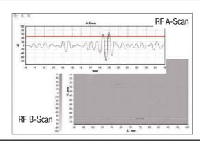
To measure precisely the item thickness and defects coordinates, the undetected RF (radiofrequency) signal is used what enables to assure the measurement resolution of 0,01 mm. Two modes of the point selection on the signal oscillogram by which the measurements are taken (automatic and manual) are provided in the instrument.
