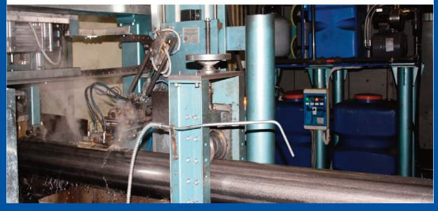
Data from ultrasonic thickness readings are collected and supplied to a computer. The resulting profile or cross-sectional view of the weld area is displayed on the graphics display.
