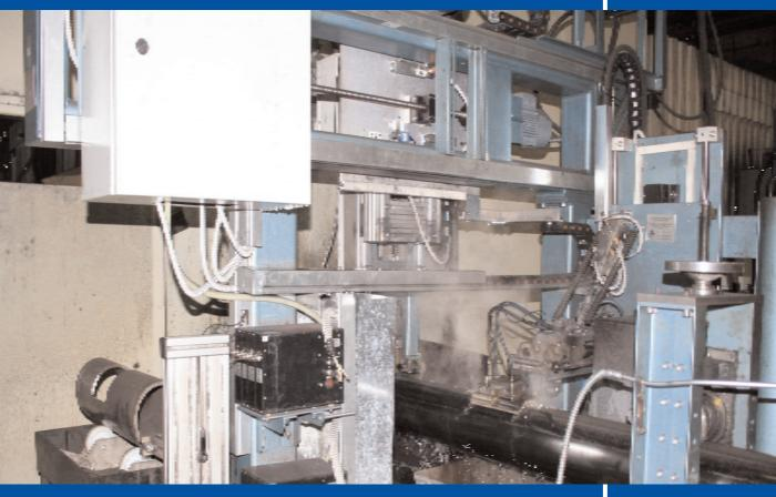
Monitoring of the ERW weld quality in in-line welding area
