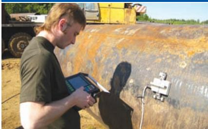
VD-OKO-01 universal multi-channel eddy current flaw detector is intended for solving a wide range of tasks of eddy current flaw detection in such branches of industry as:
