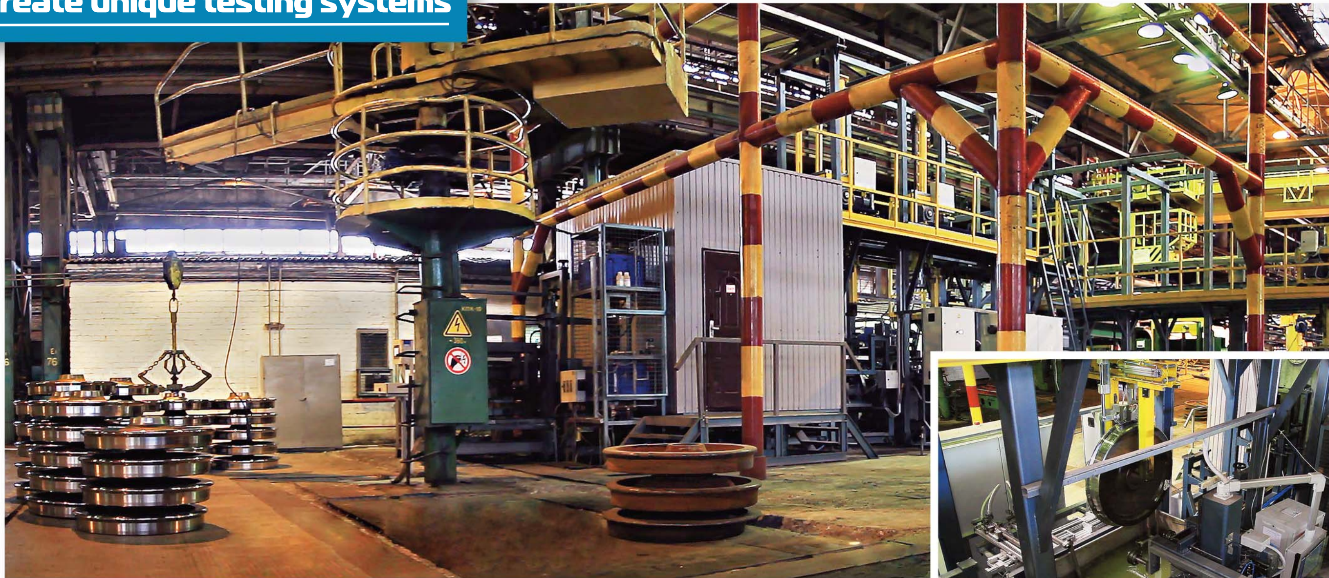
Automated line for magnetic particle and ultrasonic testing of railway wheel rim, hub, disk and flange.
