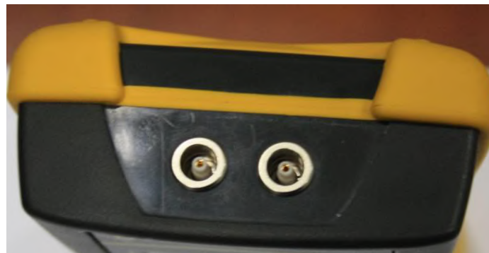
Fig. 5 – Top panel of the thickness gauge
