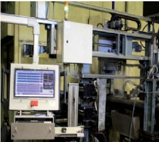
The on-line weld profile monitoring system provides the internal and external profiles of the tested weld and HAZ area along with its thickness. The material thickness and profile alarms notify the operator when the product does not meet calibration parameters. Extremely hard environment conditions are applied by IP64 OKO-22M-UT blocks. Fast Software provides high-speed tube testing with 10 channels simultaneously.
