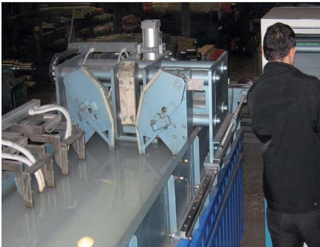
OKO-22M-UT is the best for immersion ultrasonic testing of axles and shafts for the presence of internal discontinuities and changes in attenuation of ultrasonic vibrations in the part material. The system applies all obligatory and additional techniques of acceptance ultrasonic testing, to every testing part, according to international standards. Specialized Software presents such testing results: amplitude, depth, coordinates and conditional defects sizes.
