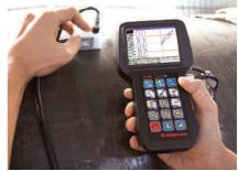
Application of VD3-81 flaw detector Eddycon for conduction of main or confirmatory body testing will enable to evaluate the pipe damage level and its further operability.
