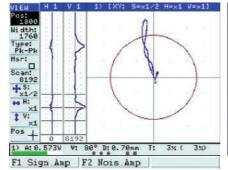
Fatigue crack 0,7 mm deep detected during testing of 18 -100 model bolster.
