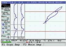
Signals of stress-corrosion defect are obtained by VD3-81 flaw detector Eddycon from the main gas pipeline section through the layer of insulation covering thickness of 6 mm.
