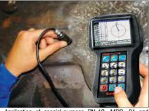
Application of special-purpose PN-12- MDP- 01 and PN-09-MDP-01 probes in protective cases together with ALARM units and digital signal processing will allow to eliminate the influence of interfering factors such as roughness, edge effect, ECP separation from the testing object surface etc.
